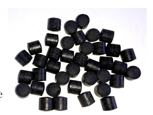
A main component 'Alumina, Silica alumina' is preferable as the carrier of ozone decomposing agent.
