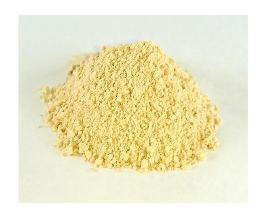
A particle size of "P-1" is set as 2 to 75  $\mu$ m, and is set at less than 200 mesh.
